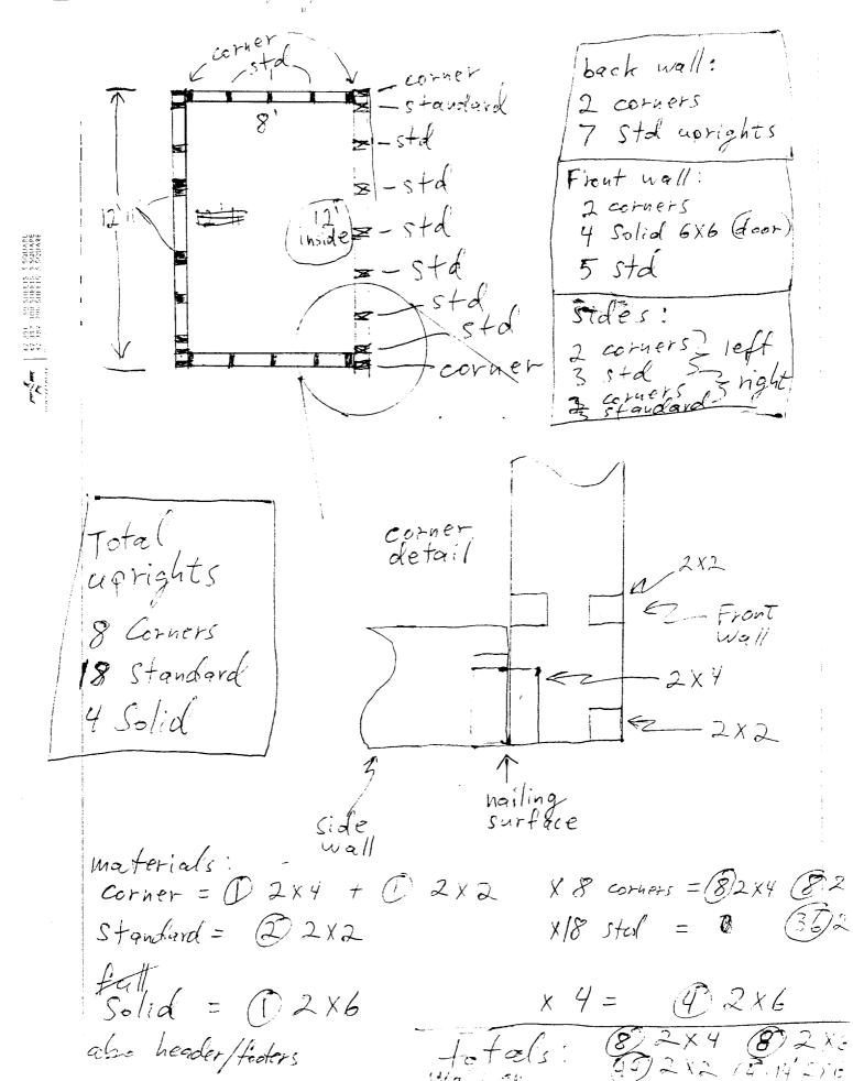
m f 2 2 x 12'11 8 2 x 4 8 8 malls: (8) 2×4 (49) 2×2 (8) 2×6 (4) 14' x 2x6 insulation- 120 linear ft 2 ft wide goop-to seal joints, tubes. 3 schews to assemble Flect: (3) 1x4 X8 Foam. High Density, hard. 1 (3) 1" 4'x8' exterior Grade Marine Ply Dinsulated door & Jam, - wide ! 6" clamps hails (15) vyny/ 4'x8' for interior strfaces
