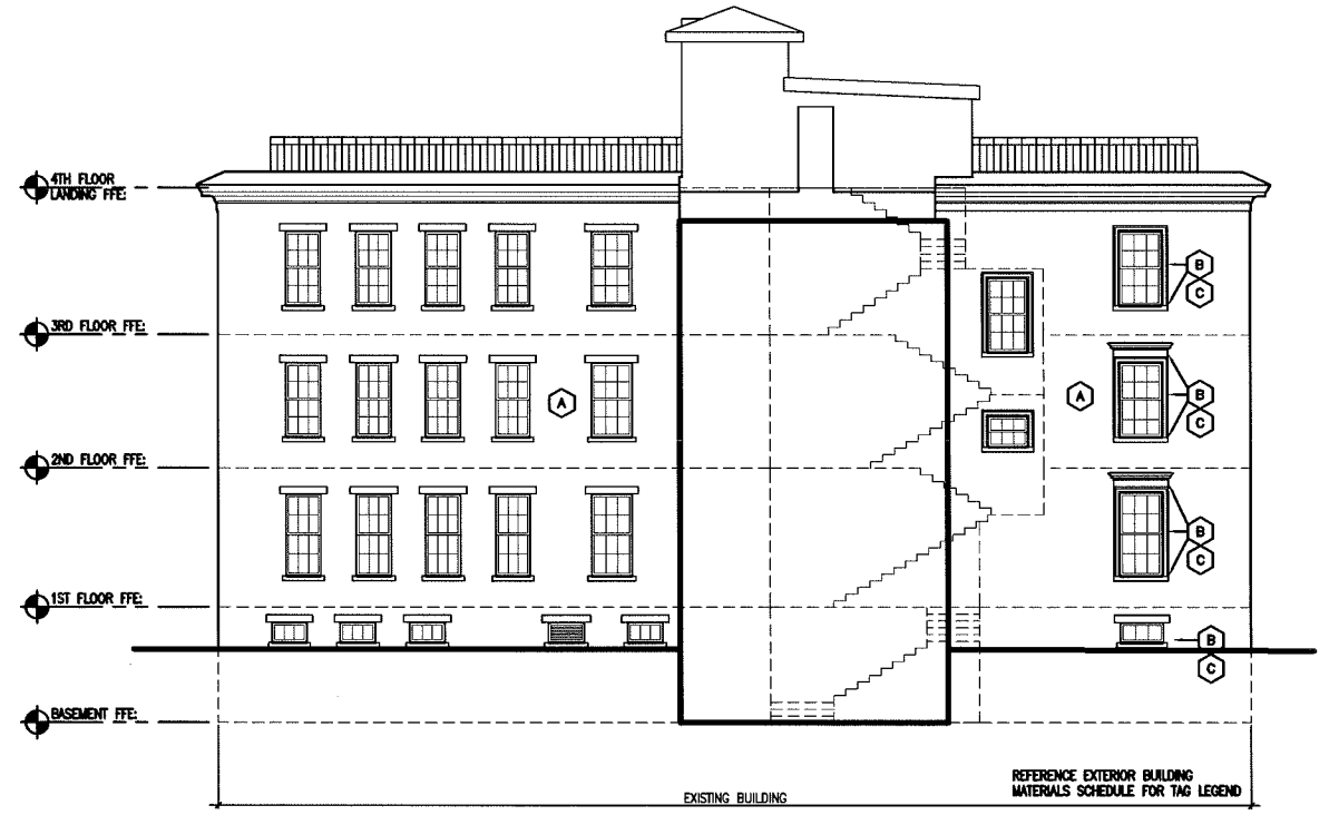
3 DANFORTH STREET ELEVATION - SECTION
