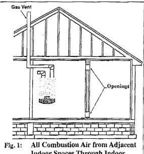
Indoor Spaces Through Indoor Combustion Openings
