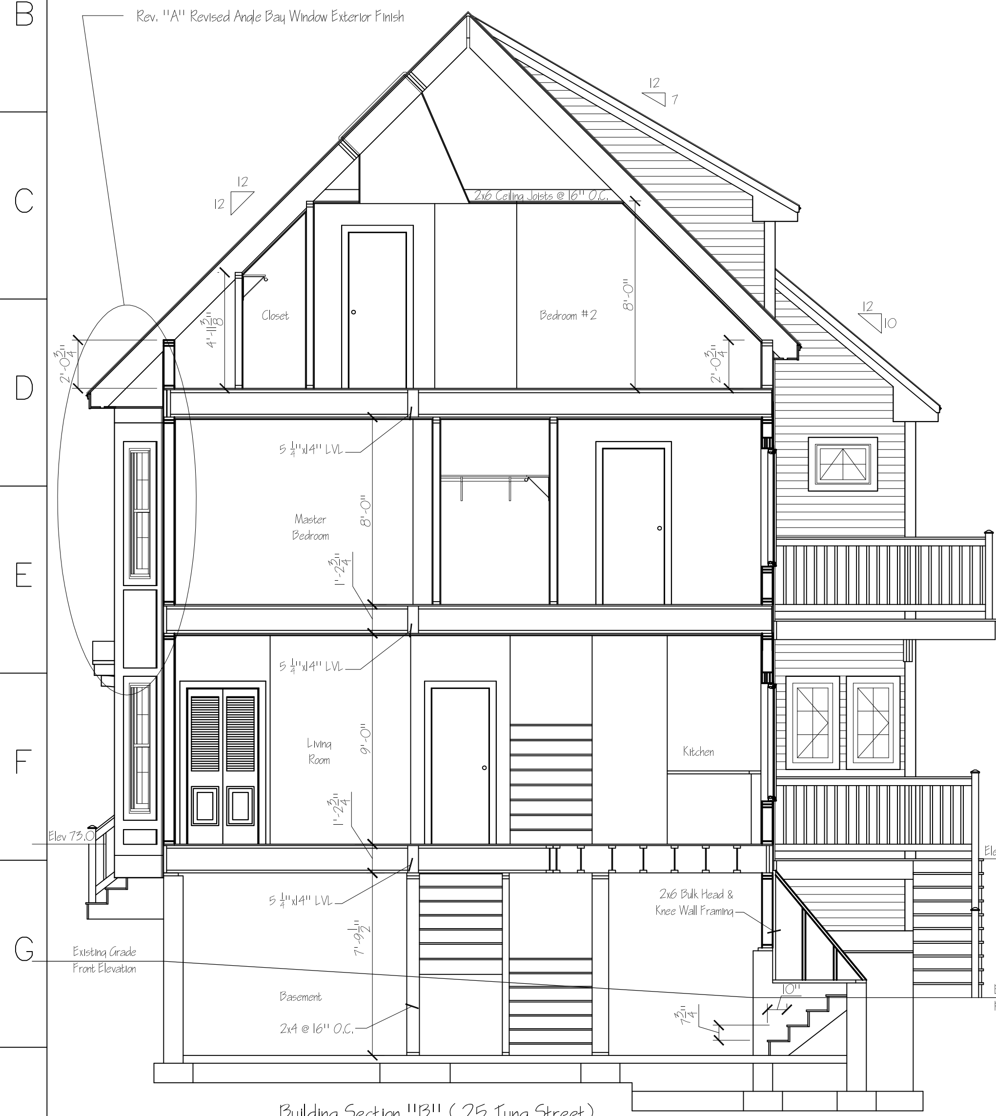
Building Section "B" (25 Tuna Street) 1/4" = 1'-0"
