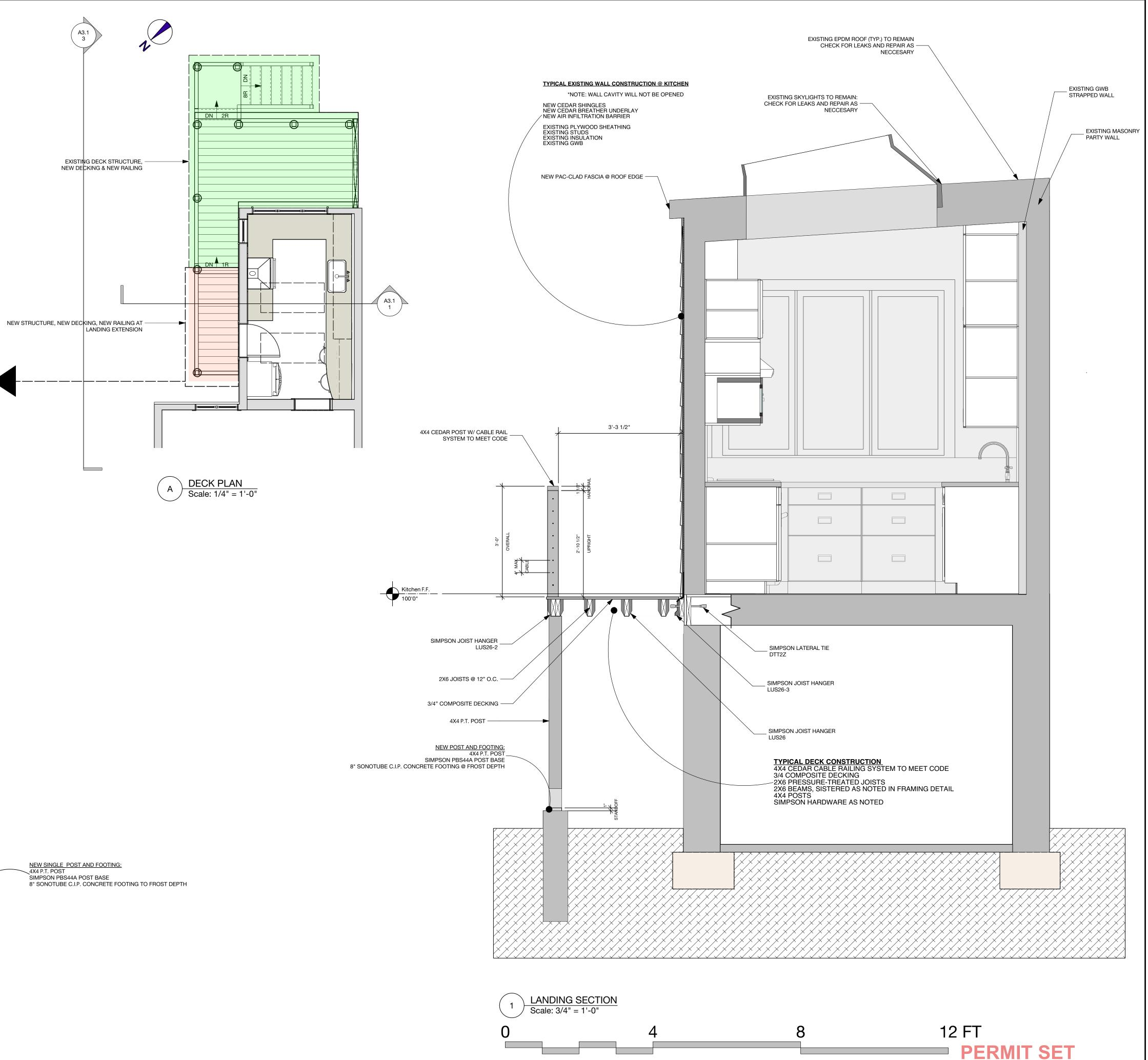
NEW SINGLE POST AND FOOTING: 4X4 P.T. POST SIMPSON PBS44A POST BASE 8" SONOTUBE C.I.P. CONCRETE FOOTING TO FROST DEPTH
