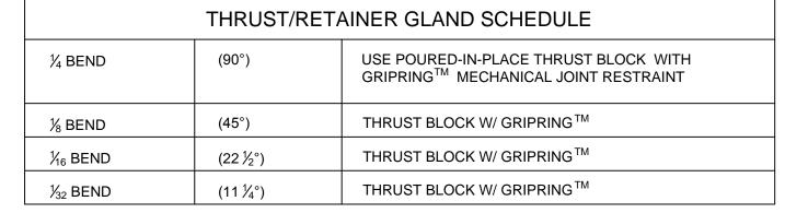
THE ABOVE SCHEDULE IS SUBJECT TO THE APPROVAL OF THE ON-SITE INSPECTOR DUE TO SOILS AND WORKING PRESSURES IN THE AREA.
