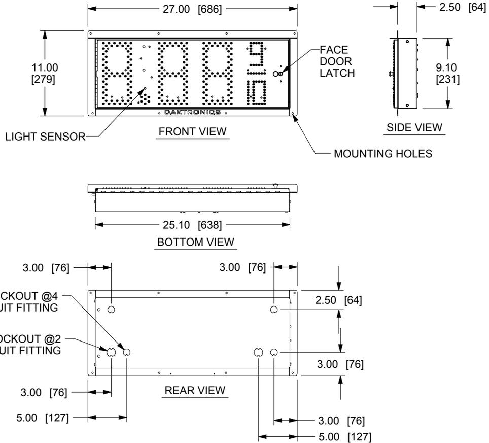
THIS IS A SINGLE FACED DROP-IN DISPLAY TO BE MOUNTED IN A RECTANGULAR OPENING IN A LARGER SIGN.
