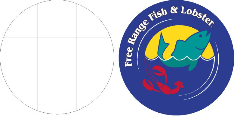
Substrate - 3mm Dibond Aluminum Composite Mounting - #10 X 1" SS Tek Screws Building - Flat corrugated steel siding
