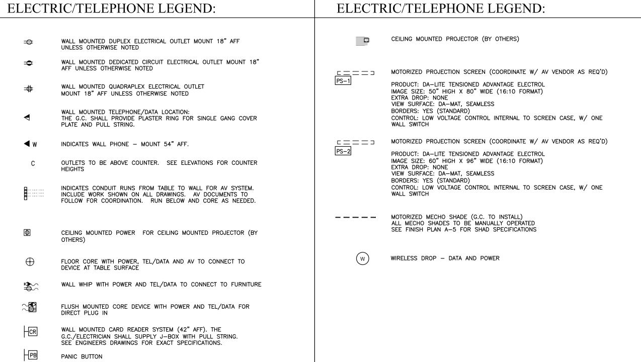
WALL MOUNTED CABLE TV LOCATION, THE G.C/ELECTRICIAN SHALL PROVIDE FROM CORE CLOSET TO LOCATION COAX CABLE AS
