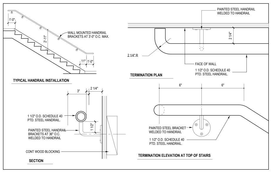
6 STAIR 1 & 2 - Wall Mounted Handrail Details
