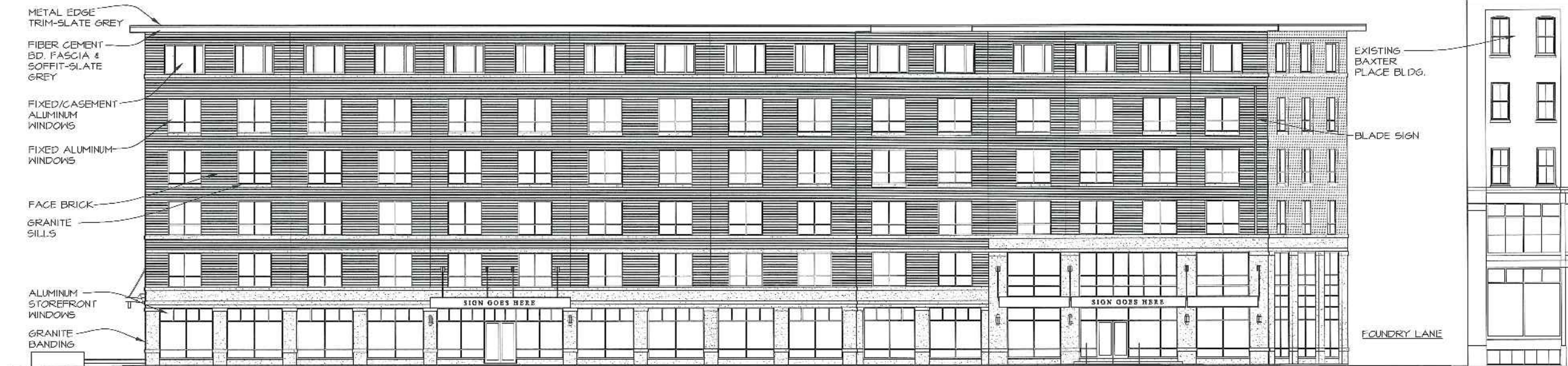
2 COMMERCIAL STREET ELEVATION C13 3/32" = 1'-0"
