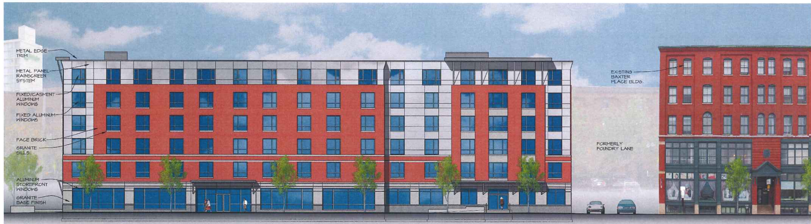
2 COMMERCIAL STREET ELEVATION 3/32" = 1'-0"
