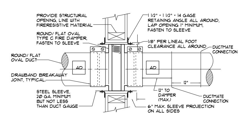
ROUND/FLAT OVAL FIRE DAMPER INSTALLATION DETAIL WHERE A 12x12 ACCESS DOOR IS NOT POSSIBLE
