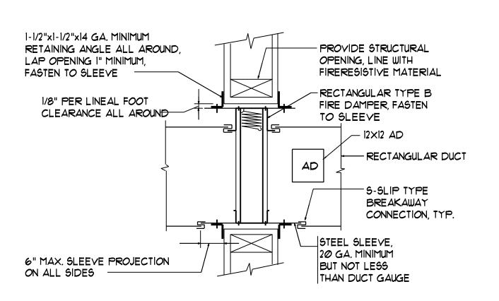
RECTANGULAR FIRE DAMPER INSTALLATION DETAIL
