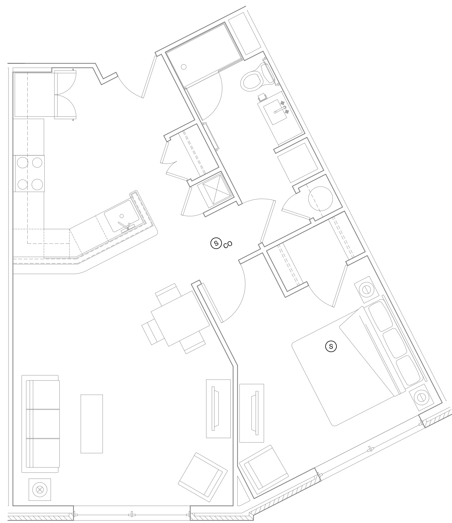
A3 1 BEDROOM UNIT FIRE ALARM PLAN 1/4" = 1'-0"; UNITS: 206, 306, 406, 506
