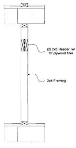
Typical Header Detail – Non load bearing walls
