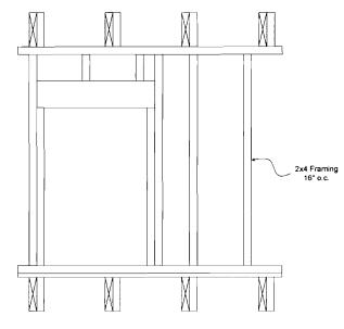
Typical Non Load Bearing Wall Framing
