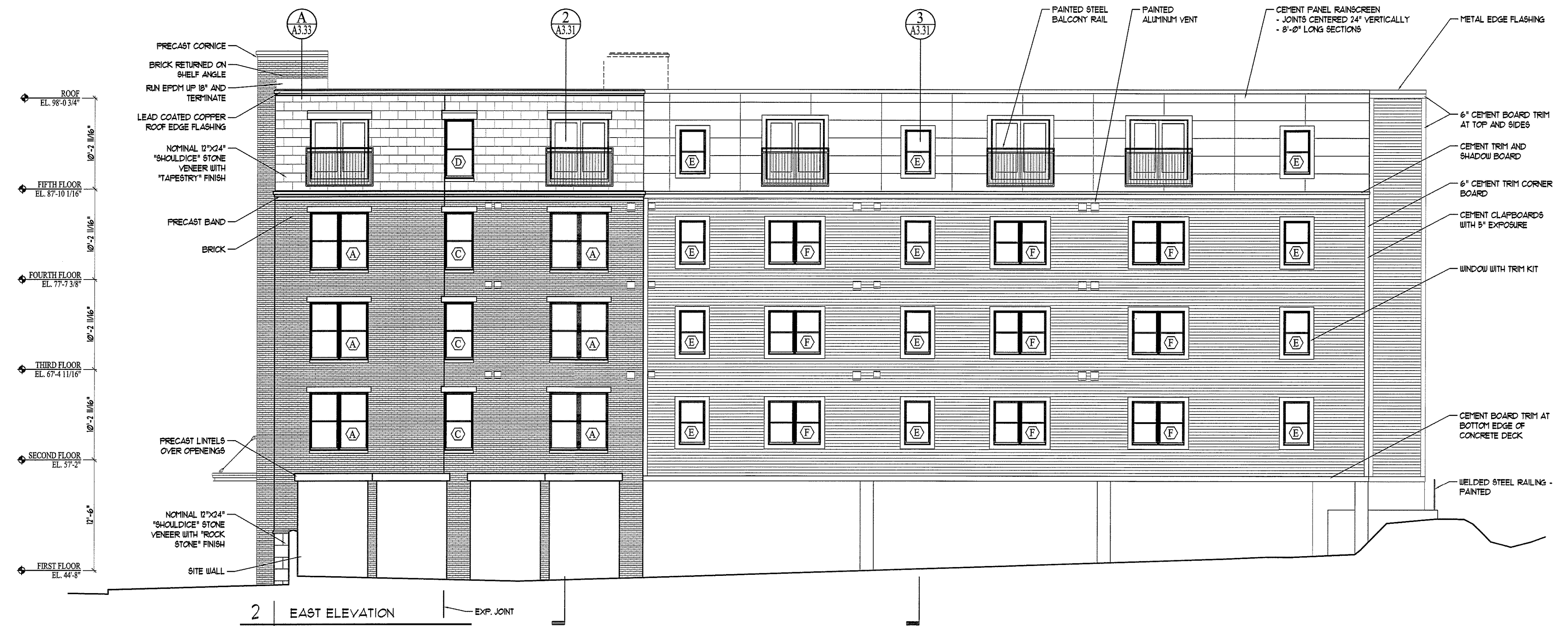
1 | SOUTH ELEVATION SCALE: 1/8"=1'-0"
