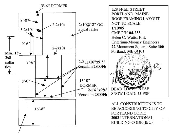
LOWER ROOF RAFTER: 2x10 @12"OC or 2x12@16"OC
