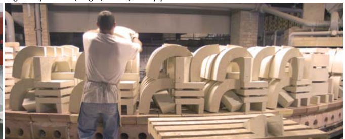
High-temperature firing of the refractory parts.
