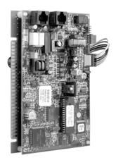
MDACT - Multi-Point Digital Alarm Communicator Transmitter
