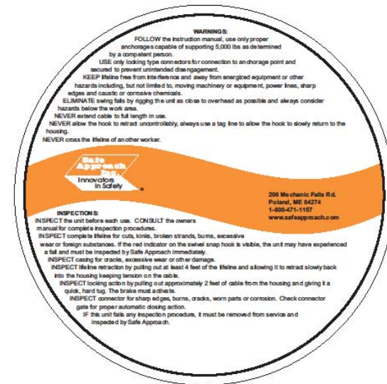
Figure 10.2: Located on back housing
