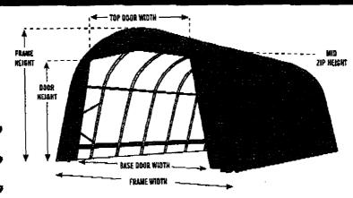
100% Galvanized Steel - We use only high yield USA manufactured carbon steel for ultimate durability, rust protection and superior strength. Each tube undergoes a triple-coating process inside and out that leaves no naked metal exposed to the elements.
