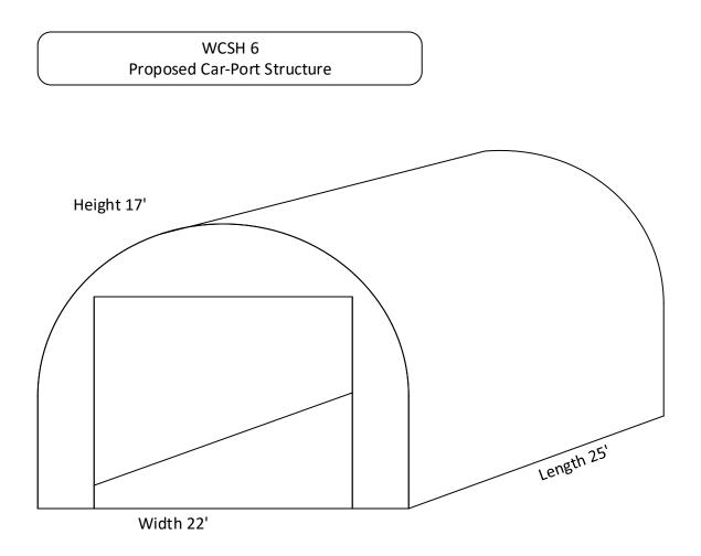
Structure is prefabricated. Made of tube steel for frame and covered in a vinyl fabric. Secured to the pavement with anchors driven into the asphalt and tied to the tube frame. Front opening has a zipper closure. Two Live News Vehicles will be kept inside. Gives protection from ice and snow.
