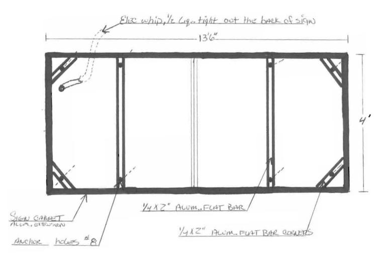
ALC ALUM ... IS WELDED 100% CABINET WILL BE ATTACKED USING 4" MILLIONALLY Steares Anchor's . Total # OF Anchors 8 fave IN CORNERS, Far IN MUDLE.
