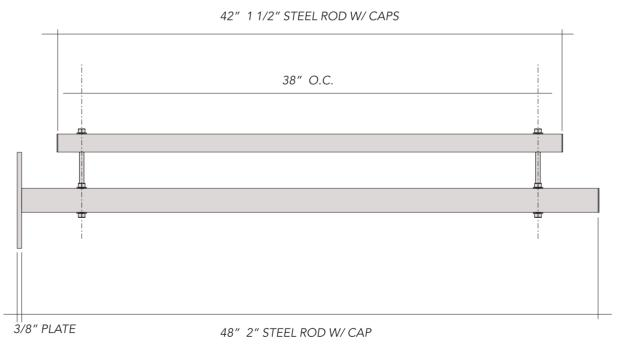
INDIVIDUAL BANNER CONSTRUCTION (2) S.F. BACK TO BACK BANNERS WITH CUSTOM PRINTS 190Z. 3M PANAGRAPHICS III FLEXIBLE BANNER MATERIAL WITH BLOCK OUT FILLER (TO ELIMINATE GHOSTING) STITCHED SIDES AND REINFORCED POLE HEMS TOP & BOTTOM WIND SLITS
