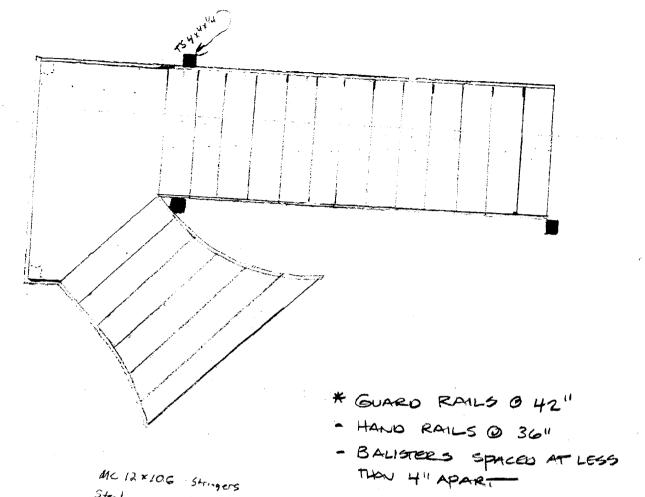
MC 12 × 106 Stringer Steel pan stair 75 4 × 4 × 4 Supports Steel balister rails Pipe Wall rails
