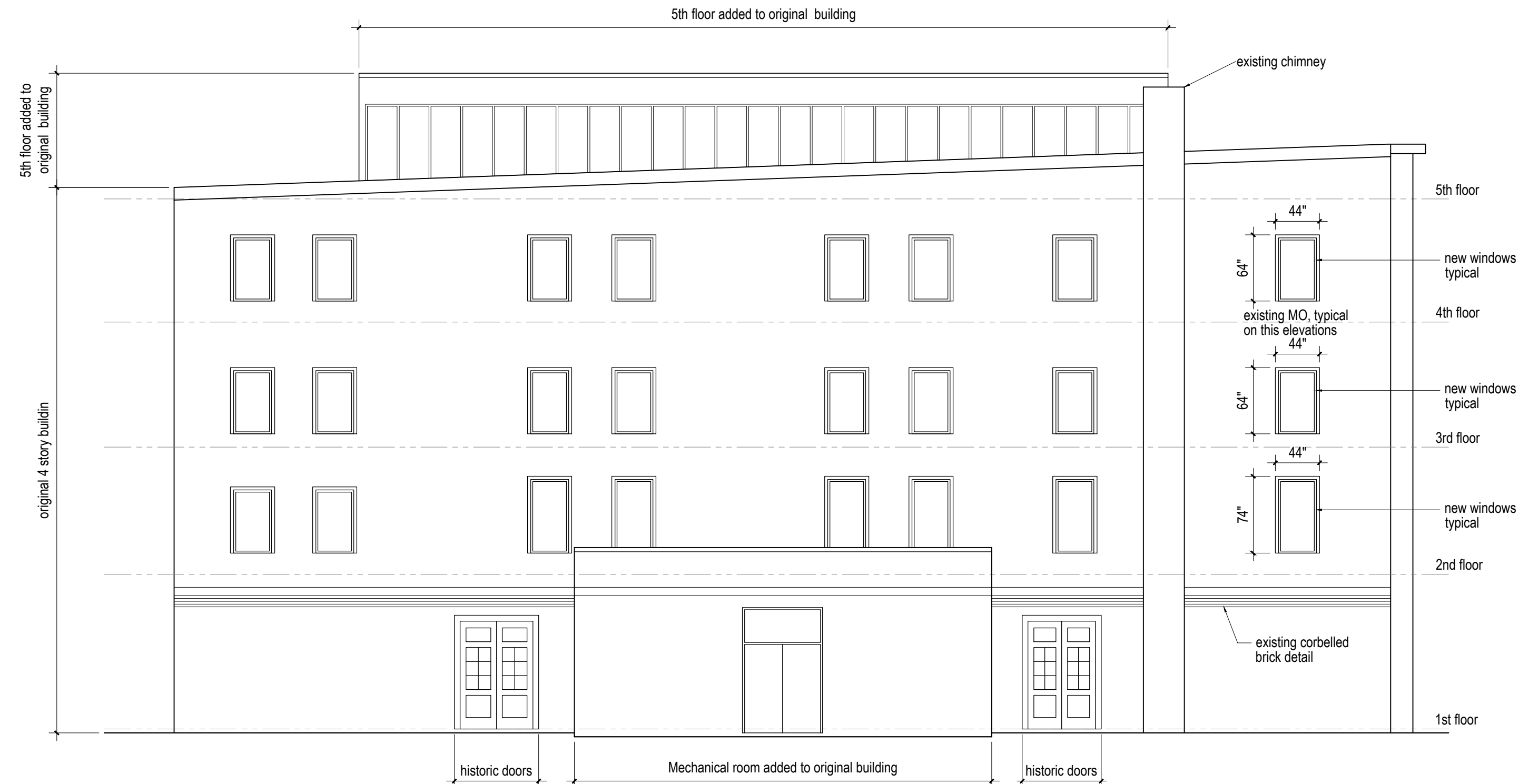
Cross Street Building Elevation: Proposed window replacement 1/8"=1'-0"
