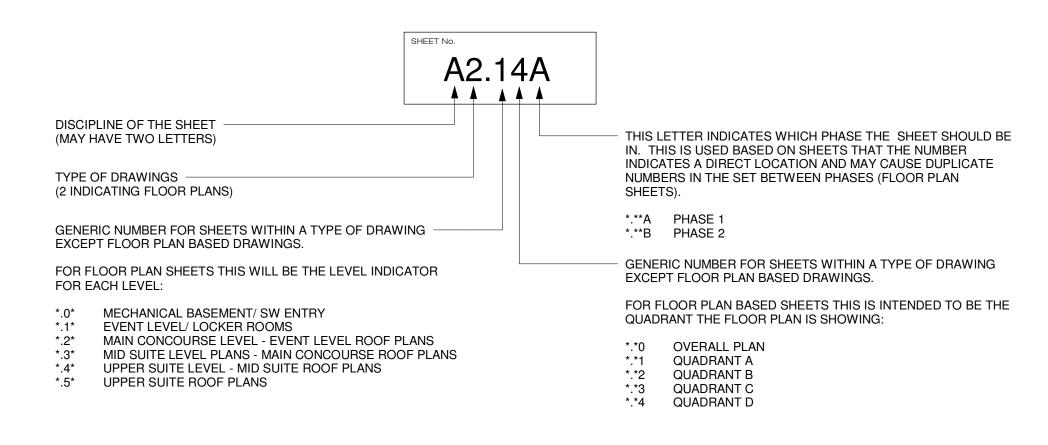
THIS DIAGRAM IS INTENDED TO BE A GENERAL GUIDE TO THE SHEET NUMBERING IN THE PROJECT, SPECIFICALLY THE FLOOR PLAN SHEETS. THIS WILL WORK WITH THE MAJORITY OF THE SHEETS WITHIN THIS SET.
