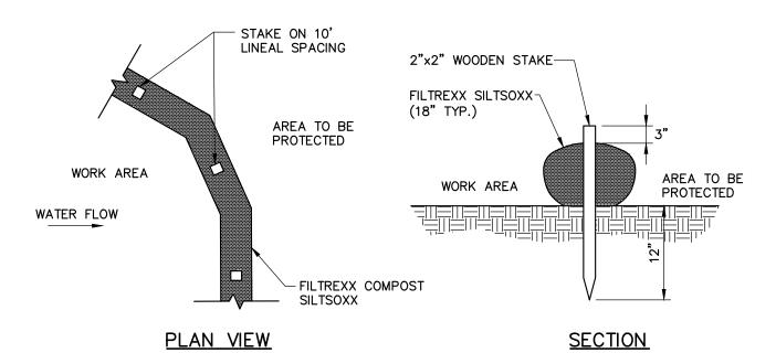
WHEN STAKING IS NOT POSSIBLE, HEAVY CONCRETE BLOCKS SHALL BE USED BEHIND THE SEDIMENT CONTROL TO HELP STABILIZE DURING RAINFALL/RUNOFF EVENTS.
