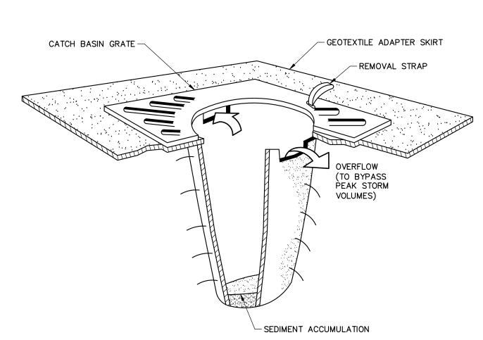
CATCH BASIN PROTECTION TO BE "SILTSACK" (BY ACF ENVIRONMENTAL) OR "STREAM GUARD" (BY FOSS ENVIRONMENTAL SERVICES). INSERT TO BE EMPTIED IN AN APPROVED MANNER WHEN IT IS 1/2 INSPECT INSERT AFTER ALL RAINFALL EVENTS, REPAIR AND MAINTAIN
