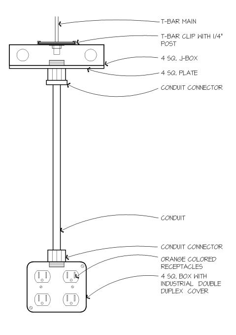
4B DETAIL @ ELECTRICAL DROP AT BACK SIDE OF RACK A401 / SCALE: N.T.S.
