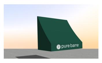
EXISTING AWNING. RECOVER WITH NEW FABRIC USING EXISTING FRAME AND ATTACHMENT POINTS
