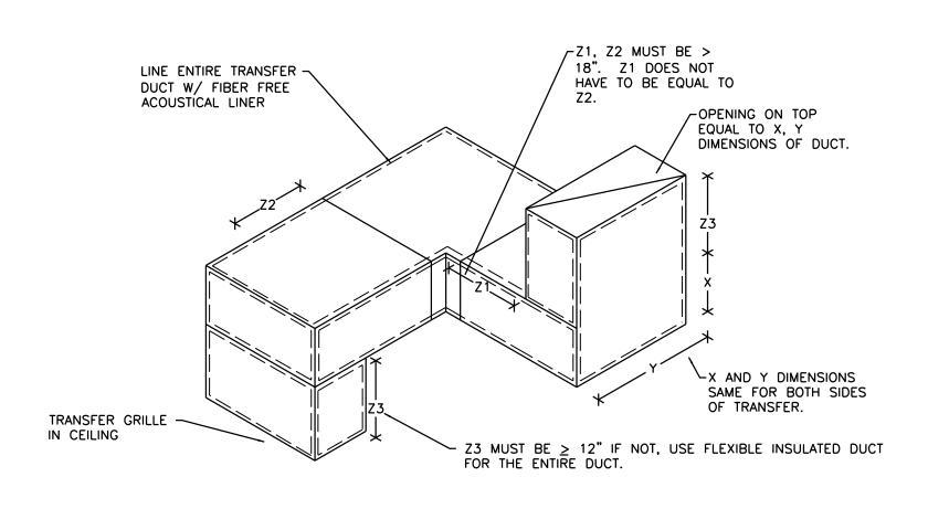
3 TRANSFER DUCT DETAIL (SPEECH BAFFLE)
