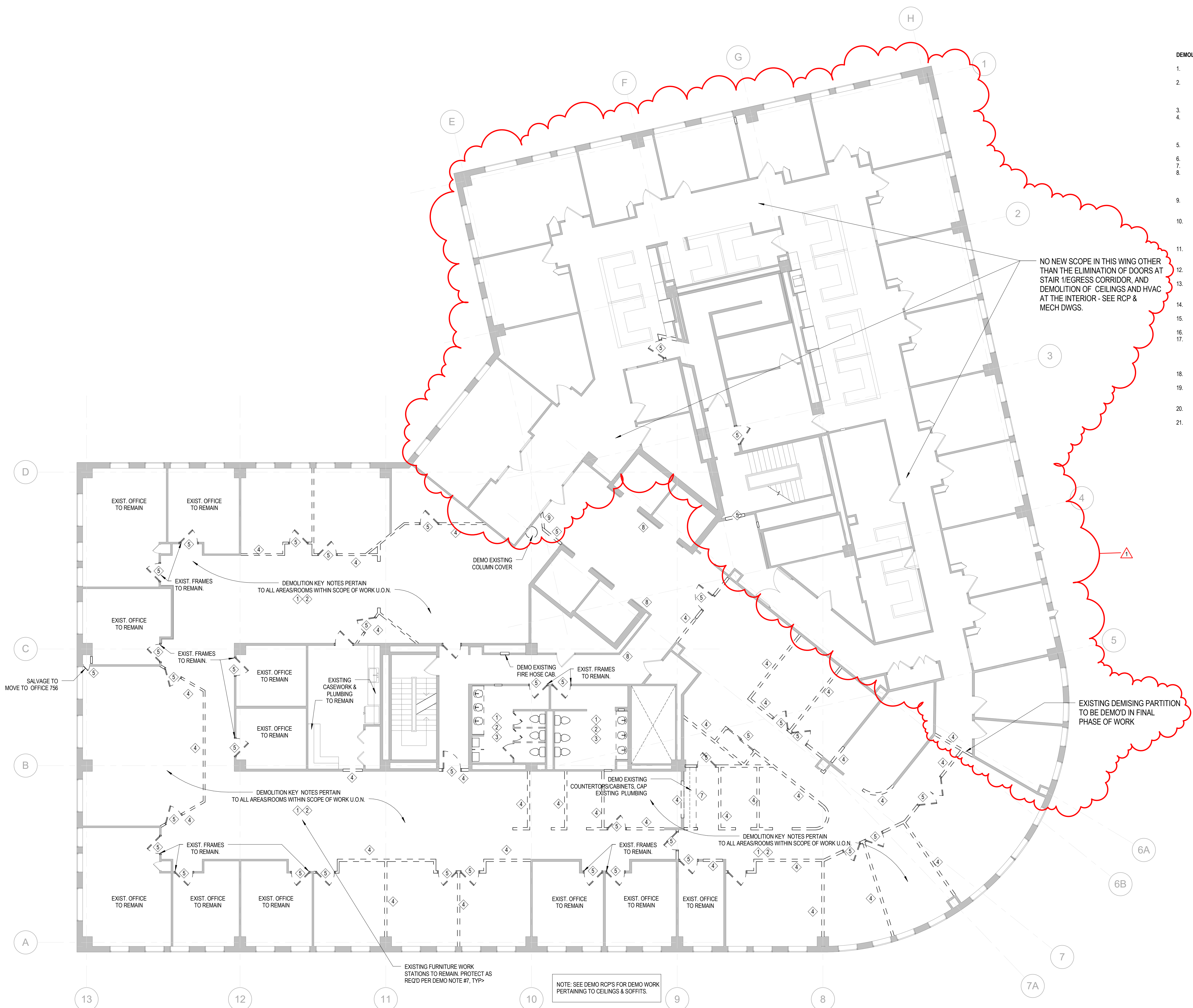
1 SEVENTH FLOOR DEMOLITION PLAN 1/8" = 1'-0"
