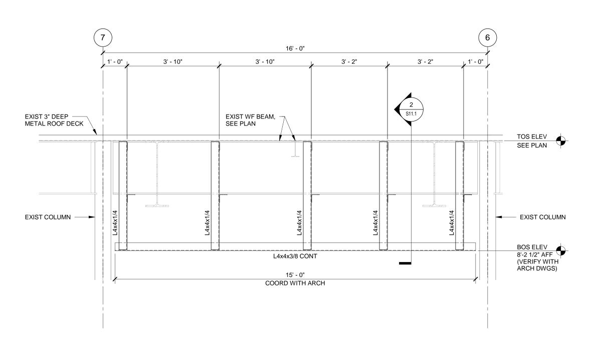
1 NANAWALL #10-01D SUPPORT FRAMING ELEVATION SCALE: 1/2" = 1'-0"
