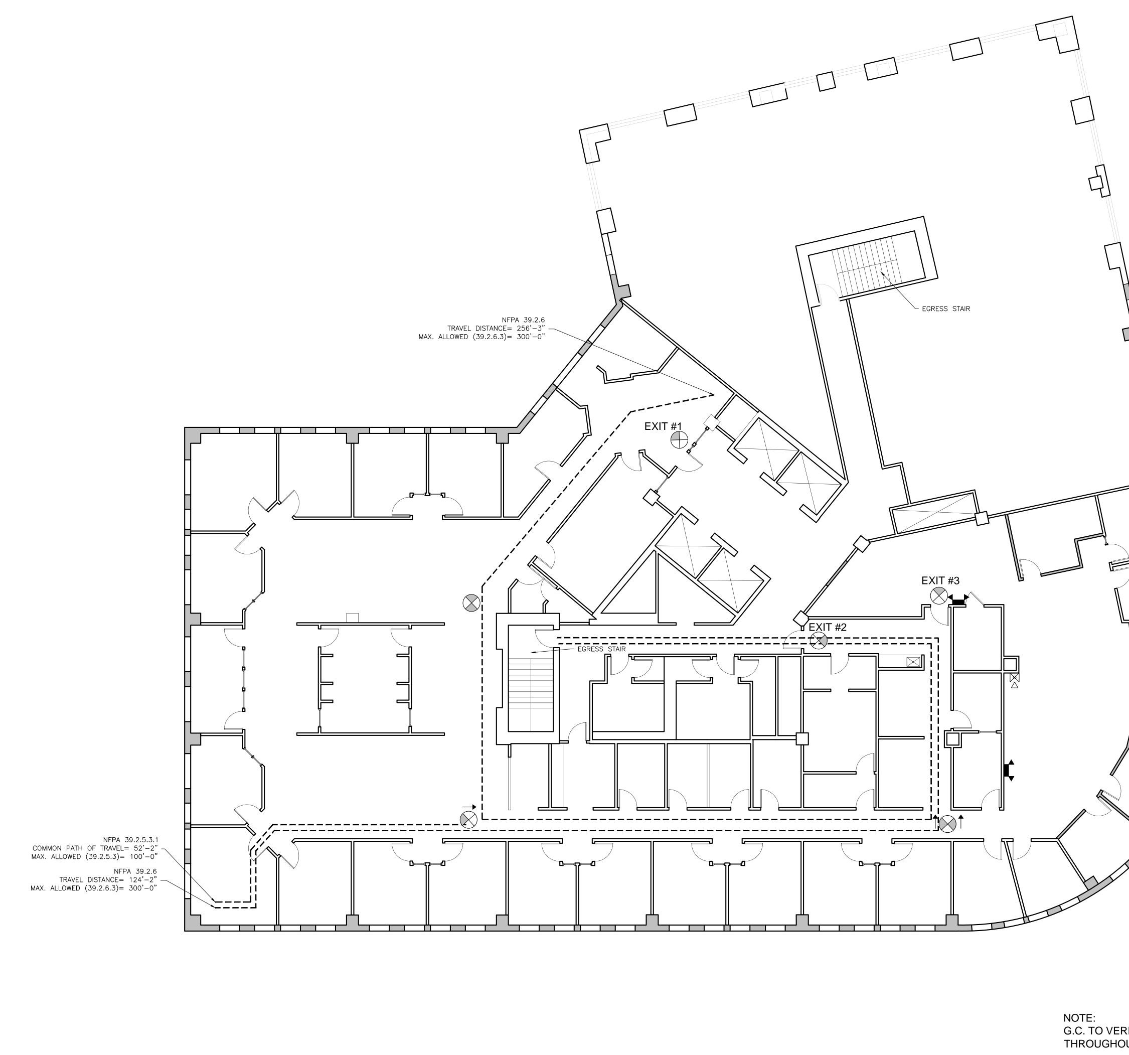
1. OCCUPANCY LOAD - MEANS OF EGRESS IBC CHAPTER 10 (CALCULATION ARE FOR THE EGRESS WITH THE OCCUPIED SPACE) DESIGN TOTAL FOR BUSINESS (B) USE CLASSIFICATION = 100 GROSS
