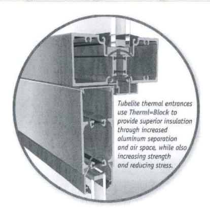
Tubelite ThermI=Block Entrances are designed using the same durable components as our Standard Entrances for outstanding craftsmanship and strength, with the additional benefit of maximum insulating properties. The Medium Stile Door has a face dimension of 4" and is designed for typical commercial use with a greater variety of hardware options. Bottom rail height is 10" for accessibility requirements. Snap-in glass stops provide for 1" glazing thicknesses.
