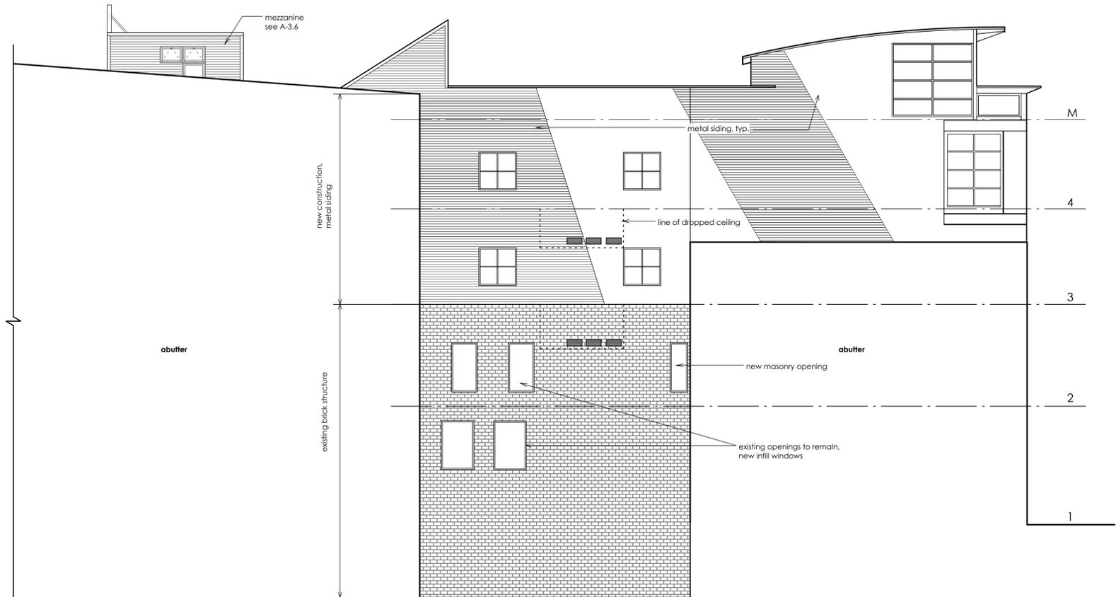
AIRSHAFT (EAST ELEVATION)
