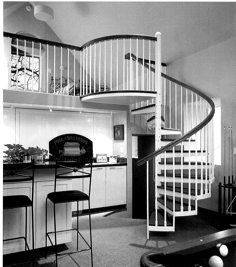
(Left) 6'0" Diameter Standard Metal Kit (22 1/2° treads) with optional oak tread & special shaped landing coverings, solid oak handrail with finger groove (Design A), double in-between spindles, continuous sleeves, closed tread ends, special shaped landing, dome center pole cap, and custom well railings with matching oak top. (Stair painted and treads & handrail stained by owner.) Robert A. Gilmour
