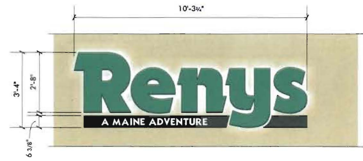
INTERNALLY ILLUMINATED HALO-LIT LETTERS & LOGO W/ FACE-LIT TAGLINE BOX SCALE: 3/8"=1'-0"
