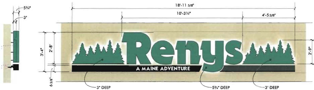
INTERNALLY ILLUMINATED HALO-LIT LETTERS & LOGO W/ FACE-LIT TAGLINE BOX SCALE: 3/8\" = 1'-0\"
