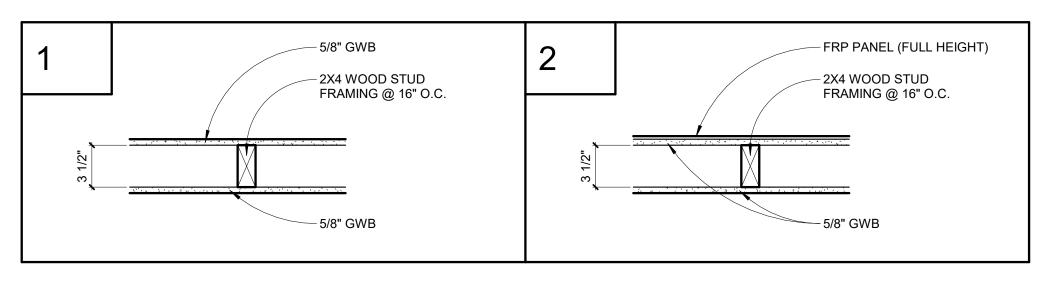
NOTE: PROVIDE MOISTURE RESISTANT GWB AND ACOUSTICAL BATT INSULATION AT ALL BATHROOM WALLS
