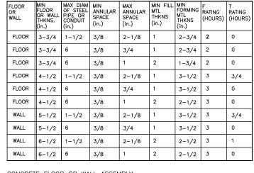
CONCRETE FLOOR OR WALL ASSEMBLY,-MINIMUM 3-3/4 in. THICKNESS FLOOR/ MINIMUM 6-1/2 in. WALL
