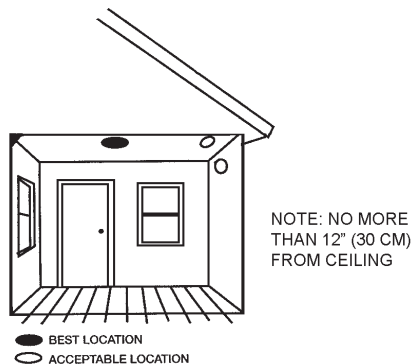
FIGURE 6: RECOMMENDED SMOKE/CO ALARM MOUNTING LOCATIONS
