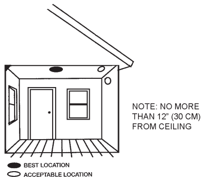
FIGURE 6: RECOMMENDED SMOKE/CO ALARM MOUNTING LOCATIONS
