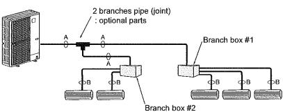
■ Installation procedure (2 branches pipe (joint))
