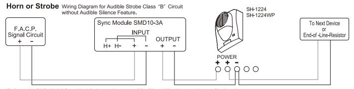
Refer to the SMD 10-3A Sync Module instruction manual for Class "A" wiring or other application diagrams.
