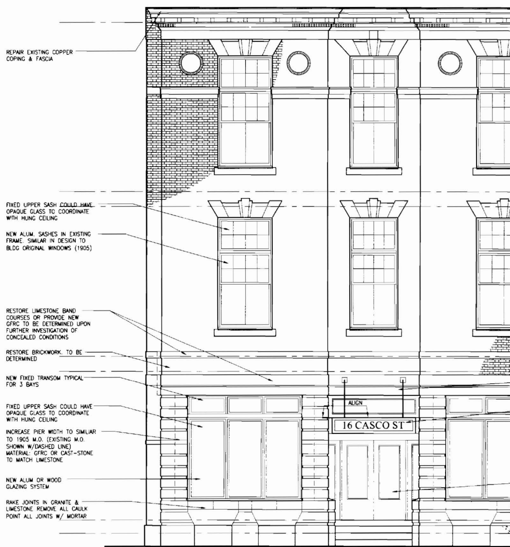
A CASCO STREET ELEVATION (EAST) 1/4"=1'-0"
