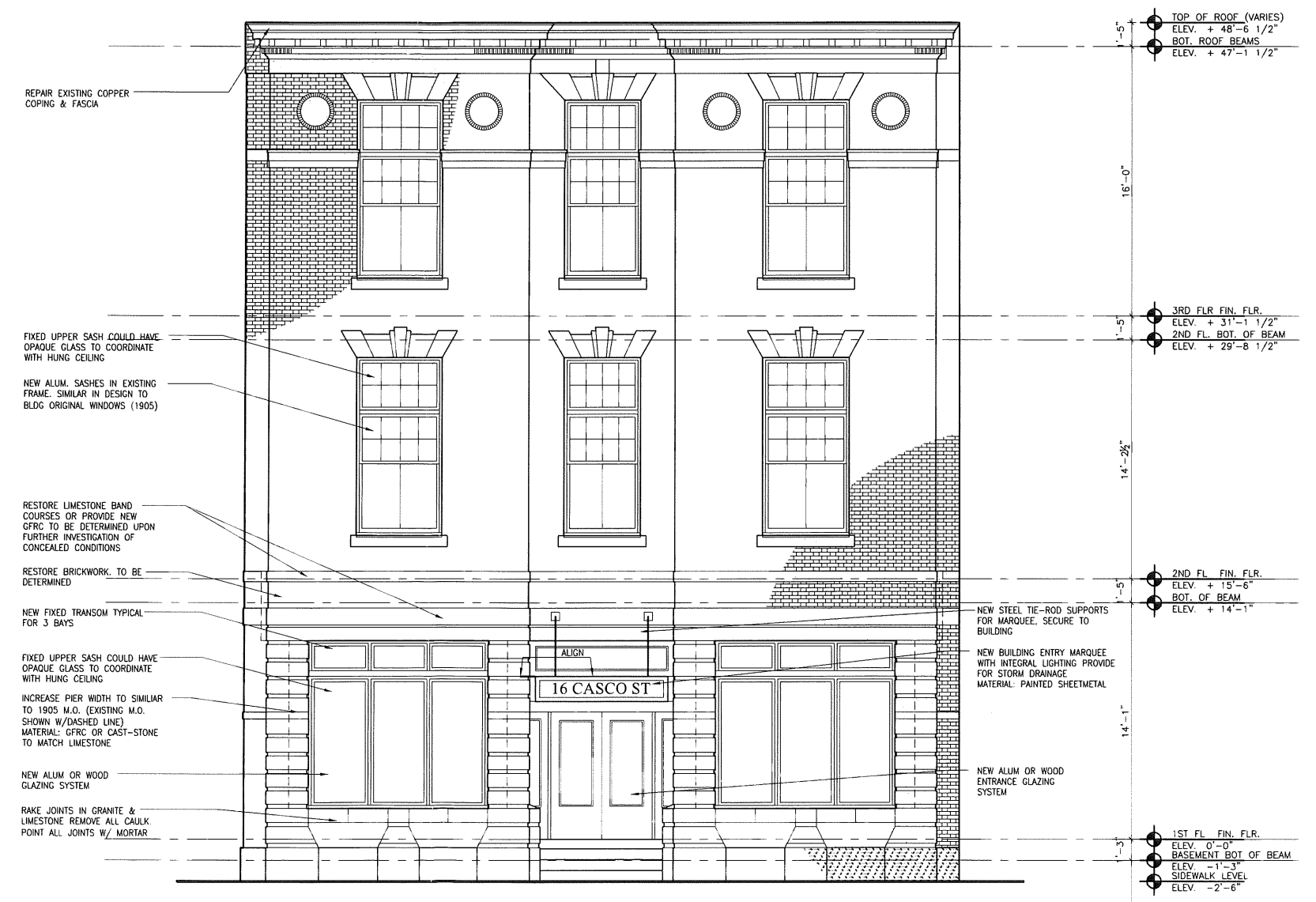
A CASCO STREET ELEVATION (EAST) 1/4"=1'-0"
