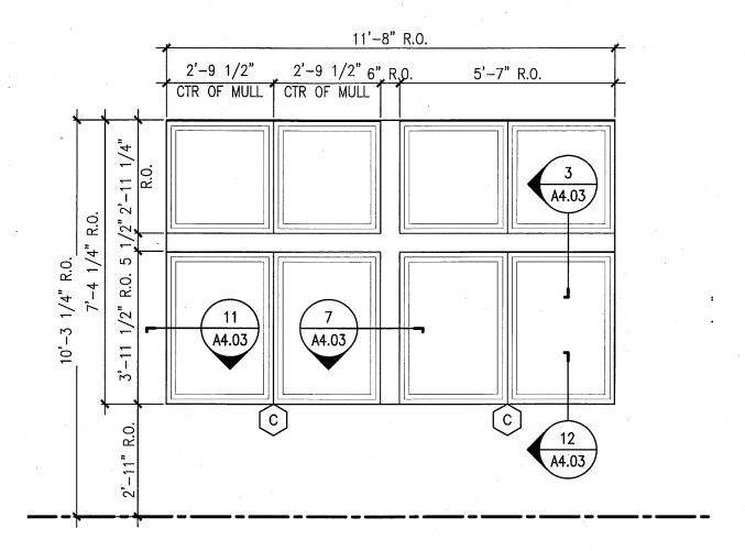
FACTORY MULLED PAIR FIBERGLASS PICTURE WINDOW SYSTEM PRE-DRILLED FOR JAMB FASTENING
