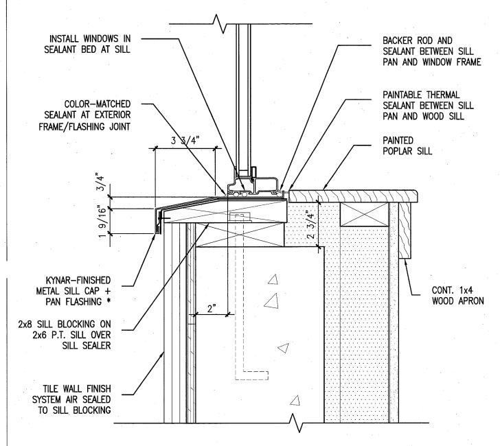
\* KYNAR-FINISHED METAL OR SINC-TIM COATED COPPER SILL CAP + PAN FLASHING WITH 1/4" UP-TURNED INNER LIP AND RETURNED EDGES (MAY BE TWO PIECES FIELD SEALED)
