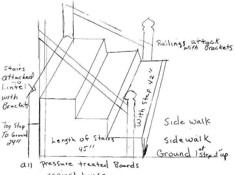
Height ground to Top Step 24" attach to The Lentel + house sides of door Jam
