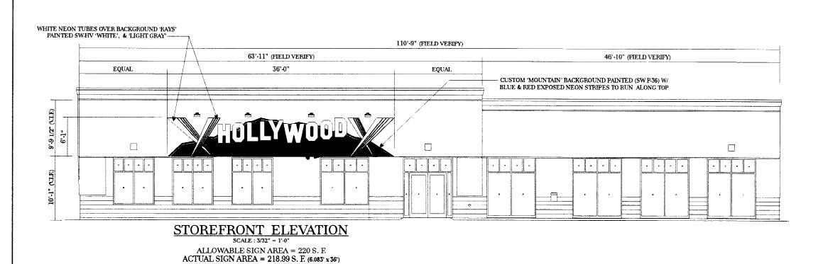
30" 'HOLLYWOOD' 15" 'VIDEO' TYPICAL CHANNEL STYLE LETTERS 'HOLLYWOOD' TO HAVE #7328 WHITE PLEXI FACE, 'VIDEO' TO HAVE #2793 RED PLEXI FACE. BOTH SETS OF LETTERS TO HAVE BLACK RETURNS & TRIM, BOTH SETS TO BE MOUNTED ON CENTER RACEWAYS. LETTERS MOUNTED ON 1/8" ALUM 'MOUNTAIN' PANEL PAINTED (SW P-36) W/ BLUE & RED EXPOSED NEON STRIPES RUNNING ALONG TOP OF PANEL. PANEL TO BE SET OFF WALL W/ SPECIAL ALUM. SPACER RACEWAY W/ ANGLE IRON FRAME. PANEL TO BE BACKLIT W/ WHITE NEON TUBING.
