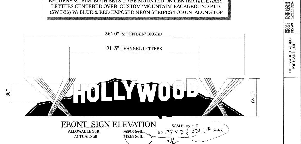
30" 'HOLLYWOOD' 15" 'VIDEO' TYPICAL CHANNEL STYLE LETTERS 'HOLLYWOOD' TO HAVE #7328 WHITE PLEXI FACE, 'VIDEO' TO HAVE #2793 RED PLEXI FACE. BOTH SETS OF LETTERS TO HAVE BLACK RETURNS & TRIM, BOTH SETS TO BE MOUNTED ON CENTER RACEWAYS. LETTERS MOUNTED ON 1/8" ALUM 'MOUNTAIN' PANEL PAINTED (SW P-36) W/ BLUE & RED EXPOSED NEON STRIPES RUNNING ALONG TOP OF PANEL.
