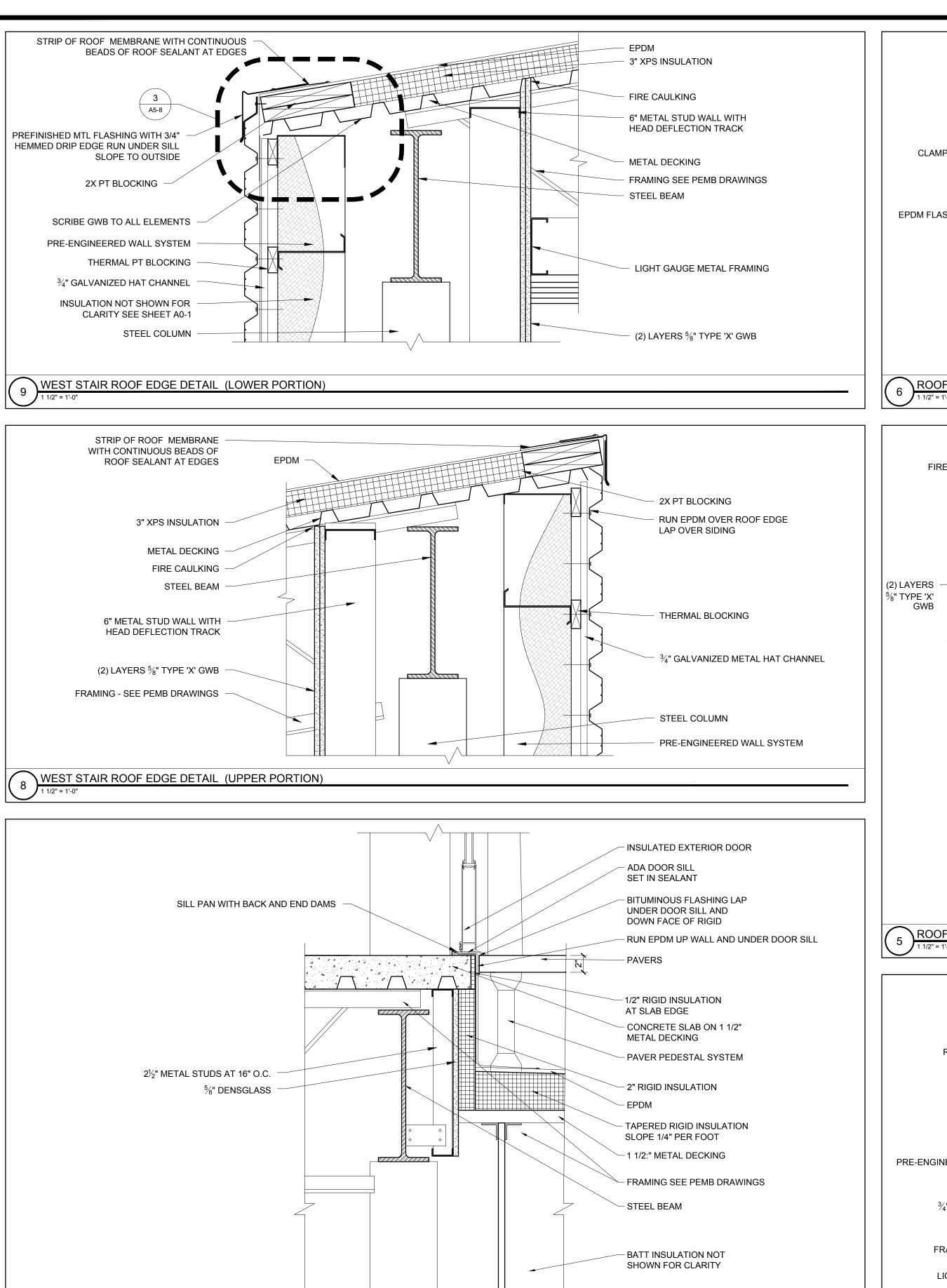
ROOF DECK DOOR SILL SECTION DETAIL
